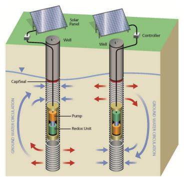
The conceptual design of the proposed solar-powered remediation strategy to reduce TCE in groundwater. Treatment units in the wells would be connected to solar panels and controllers. (Photo courtesy of Northeastern SRP)
