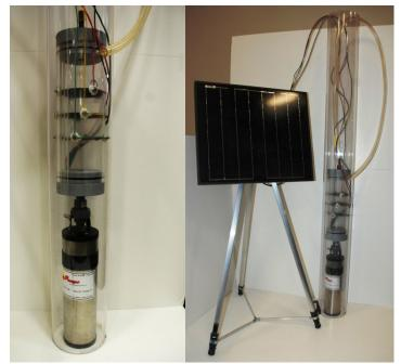
Alshawabkeh and his team have created a pilot-scale electrochemical setup to test the influence of different parameters on removal of TCE from groundwater. (Photos courtesy of Ljiljana Rajic)
