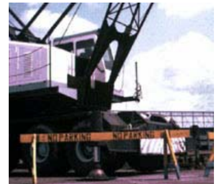
Crane swing radius guarded with barriers.
