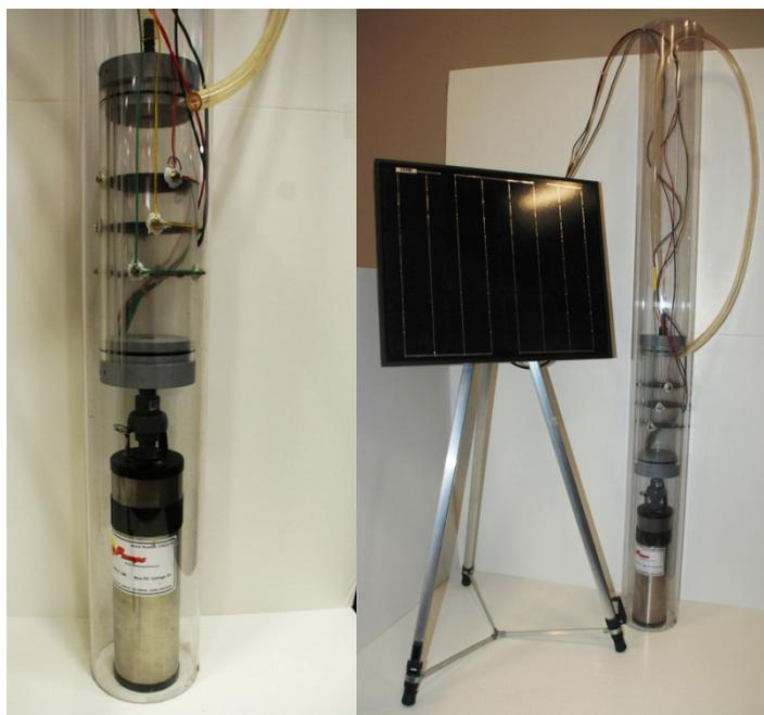
Alshwabkeh and his team have created a pilot-scale electrochemical setup to test the influence of different parameters on removal of TCE from groundwater. (Photos courtesy of Ljiljana Rajic)
