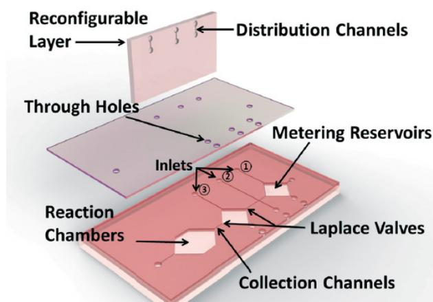
The figure above shows the structural assembly of one dilution unit in the device. The numbered inlets indicate the entry point for the diluent (1), sample (2), and reagent (3). (Image reproduced from Fan et. al. 2015 with permission of The Royal Society of Chemistry)
