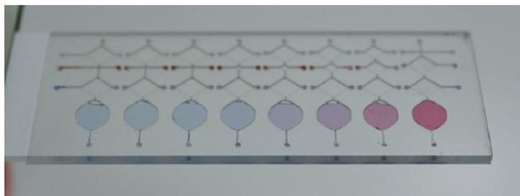
A serial dilution characterized using red dye as the sample, deionized water as the diluent, and blue dye as the detection reagent for a visual demonstration of the device. (Image reproduced from Fan et. al. 2015 with permission of The Royal Society of Chemistry)
