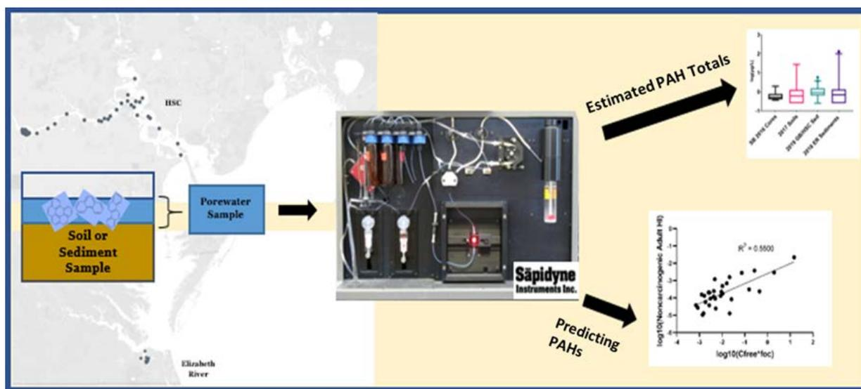
The biosensor characterizes PAH concentrations in diverse samples in real time while also serving as a predictive screening tool for potential health risks. (Image adapted from Camargo et al., 2022, Environ Res)
