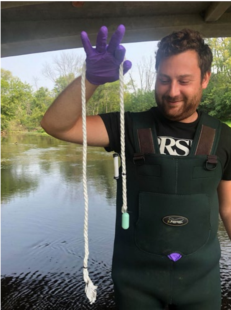
Matthew Dunn, a URI trainee under the mentorship of Center Director Rainer Lohmann, received a 2021 K.C. Donnelly Award to travel to Chicago to work with SRP-funded small business CycloPure . In this photo, Dunn uses CycloPure's DEXSORB passive sampler to measure PFAS in an urban stream.
