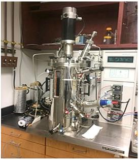
Growth of Dehalobium chlorocoercia in batch bioreactor through multiple cycles of PCE addition and purging of products.
