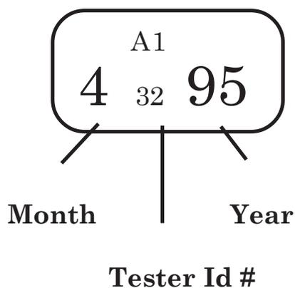
This label tells us that the bottle was last hydrostatically tested in April, 1995. Look for a mark like this on the cylinder.
