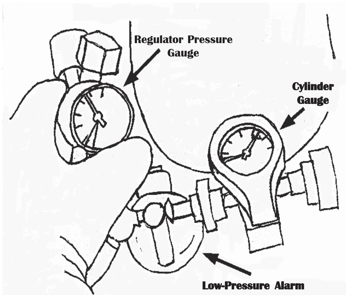
**Don't forget to check the low-air alarm and the emergency bypass valve.**
