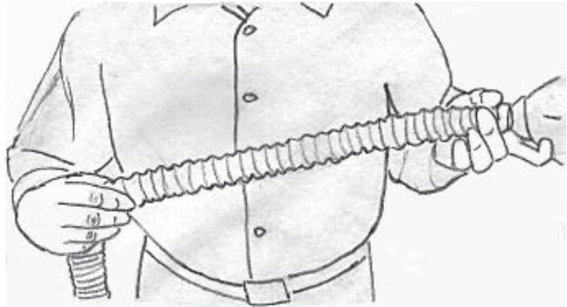
② Check the hose for leaks. Cover one end, stretch the hose and then cover the other end. Still blocking both ends, stop stretching the tube. The tube should hold the air and remain extended. If the hose collapses you have a leak.
