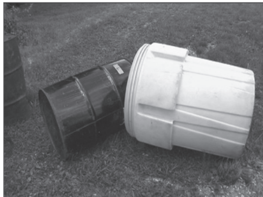
Figure 4. V-shape overpack method
