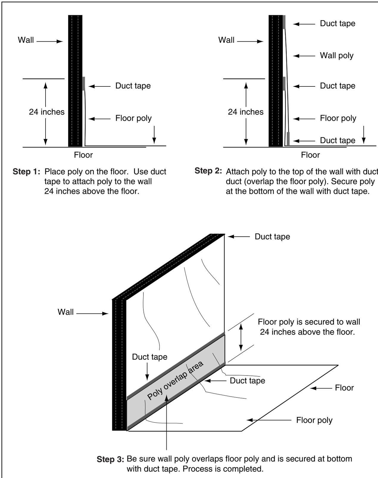
**Figure 8-3.** Follow these procedures to cover the floors and walls with poly.
