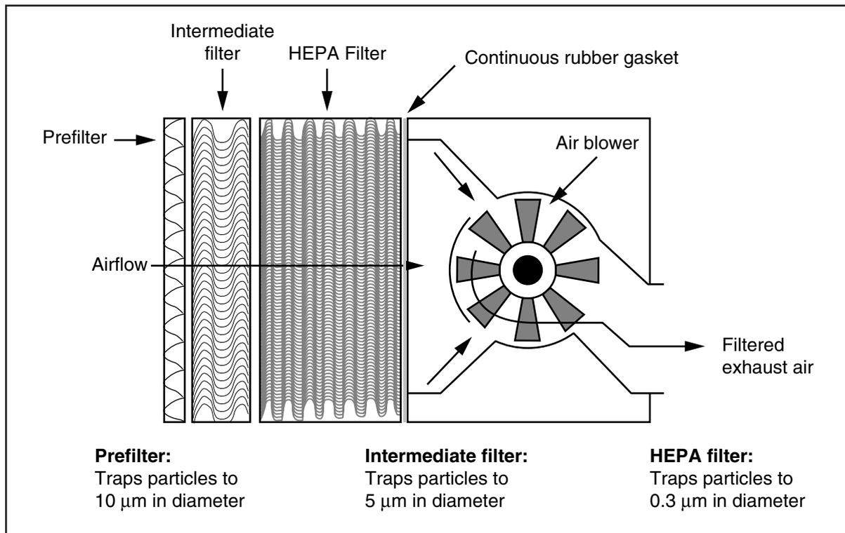
**Figure 7-2.** This figure shows a cross-section view of a HEPA-filtered exhaust fan.
