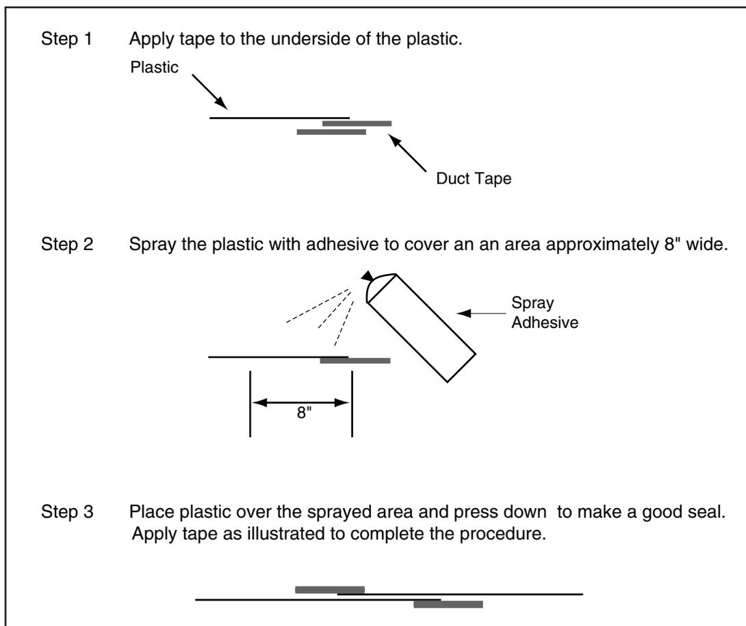
**Figure 8-2.** This figure shows the procedure for making double duct tape seams.
