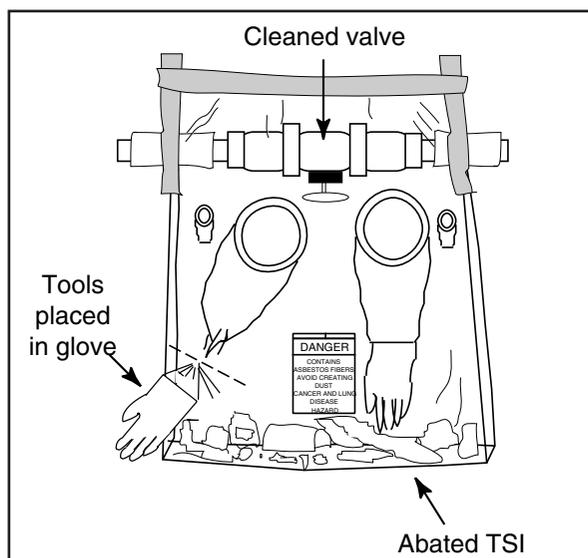
**Figure 9-5.** Invert the glove to remove tools from glove bag.
