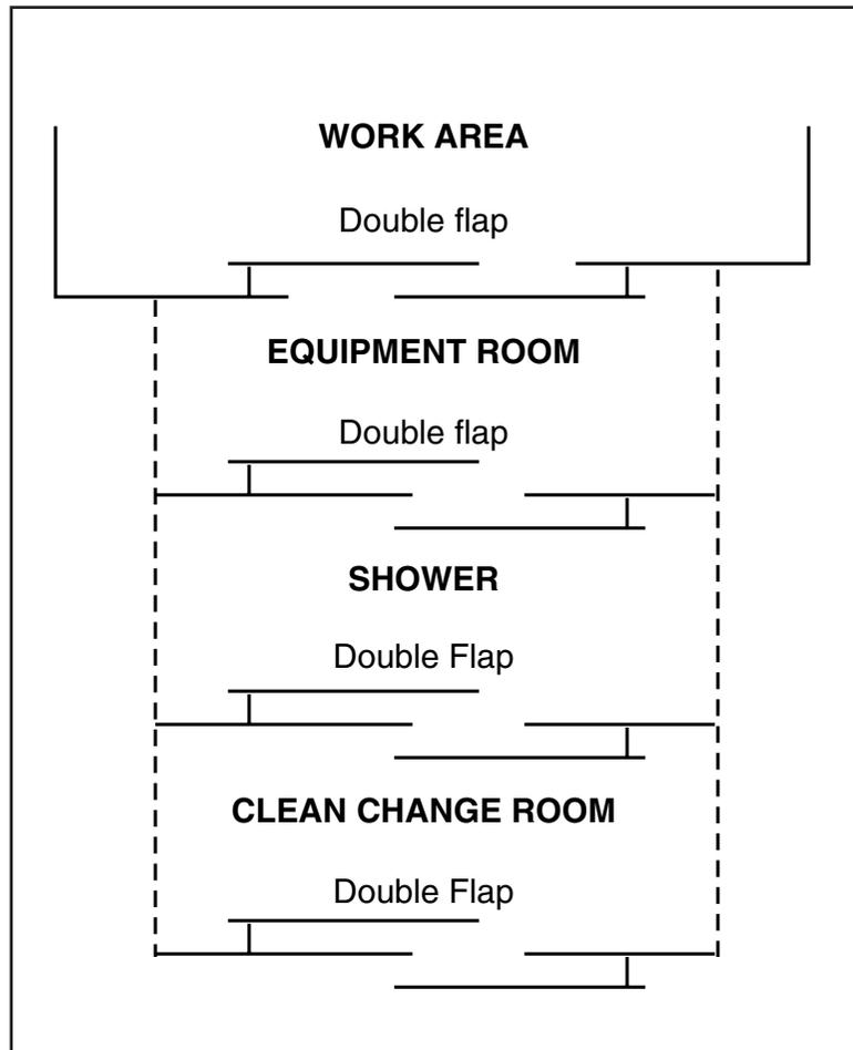
**Figure 5-14.** Workers don and doff PPE in the decontamination unit leading to the work area.
