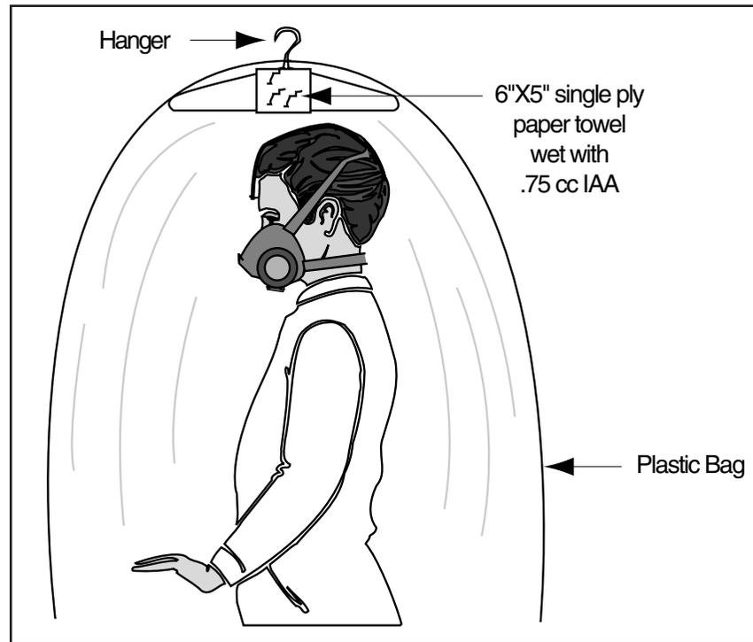
**Figure 5-13.** A fit test chamber ensures the concentration of the testing agent stays at the same level for the entire test.
