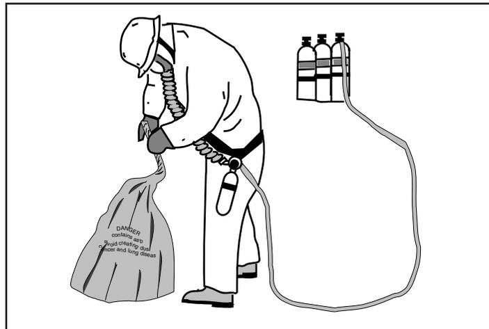
**Figure 5-9.** Air is delivered to a supplied air respirator through a hose.
