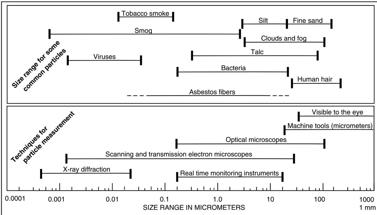
**Figure 1-2.** Size comparison between asbestos and other substances and common measurement techniques.
