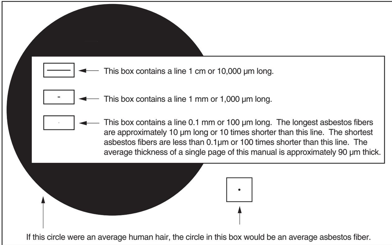
**Figure 1-1.** Size comparison between an asbestos fiber and a human hair.
