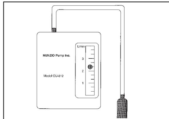
**Figure 10-1.** A personal air sampling pump used in air monitoring.
