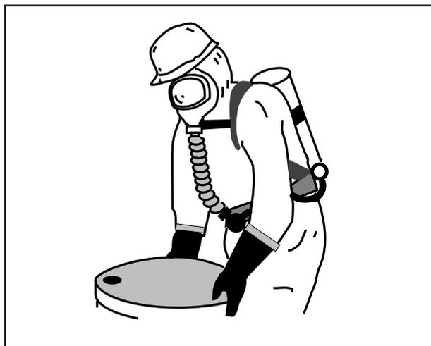
**Figure 5-10.** An SCBA receives air from a tank of compressed air.
