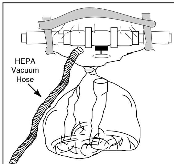
**Figure 9-6.** Collapse the glove bag with a HEPA vacuum.
