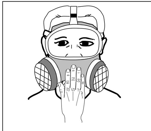
**Figure 5-11.** Positive pressure check user seal check
