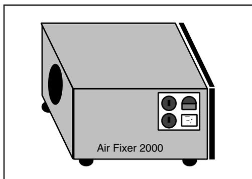
**Figure 7-1.** The HEPA-filtered exhaust fan filters contaminated air and discharges clean air.
