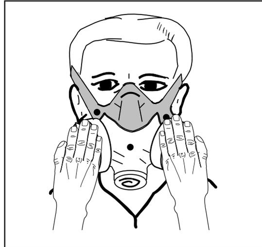
**Figure 5-12.** Negative pressure user seal check
