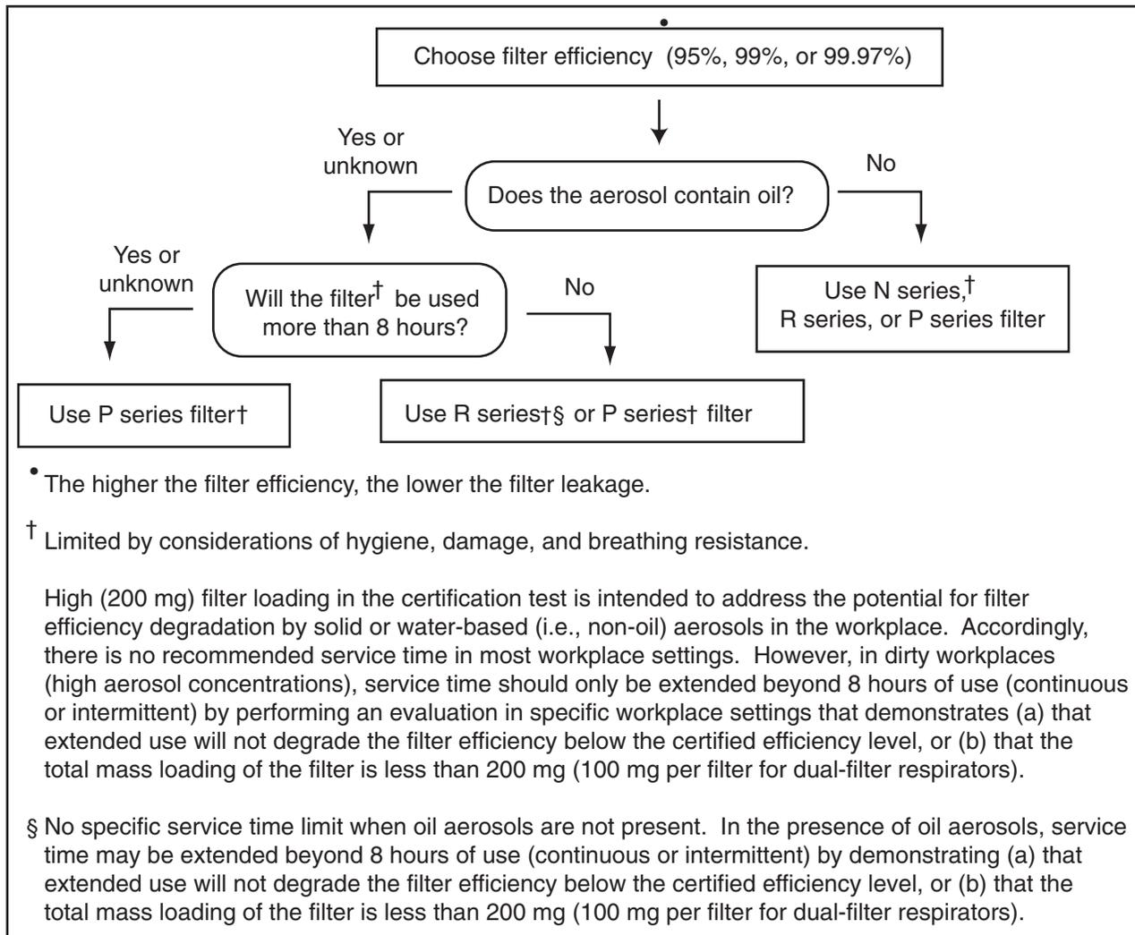
**Figure 5-8.** Flow chart for selecting Part 84 particulate filters.
