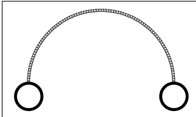
**Figure 9-1.** A bone saw has a serrated cutting wire.
