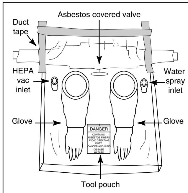
**Figure 9-3.** A typical glove bag arrangement is shown.
