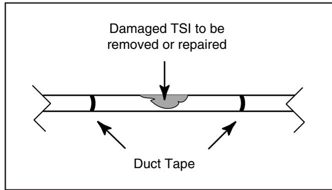
**Figure 9-4.** The pipe is prepared for glove bag attachment.
