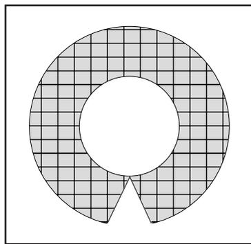
**Figure 9-2.** Cut two pieces of fiberglass cloth.
