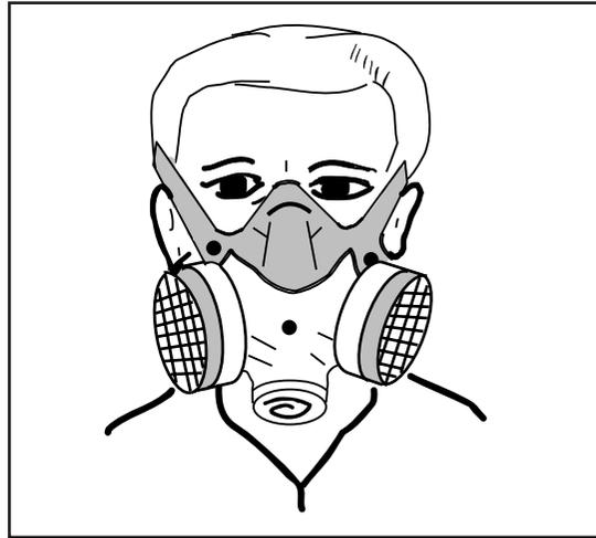
**Figure 5-3.** The half-face APR is the minimum type of respirator for asbestos abatement work.
