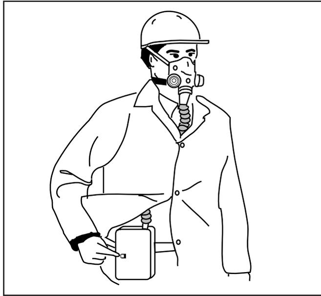
**Figure 5-5.** A powered air purifying respirator has a battery-operated blower.
