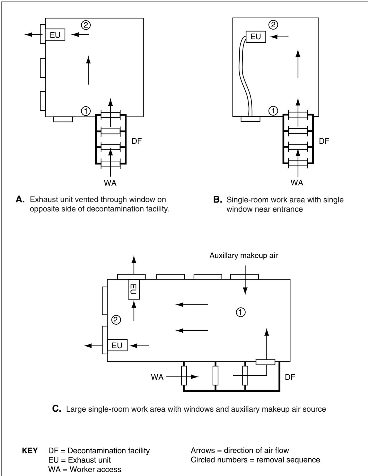
**Figure 7-3.** Three examples of negative pressure systems.
