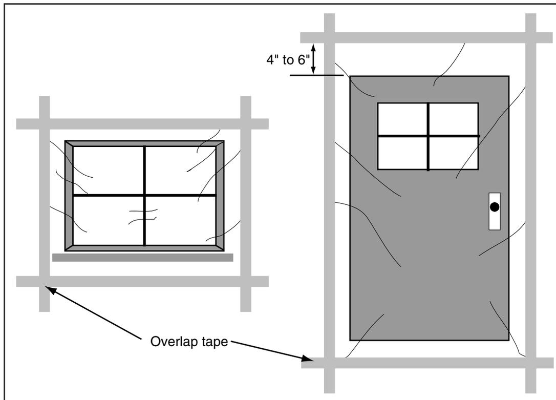
**Figure 8-1.** Windows and doors are sealed with 6-inch mil poly and duct tape.
