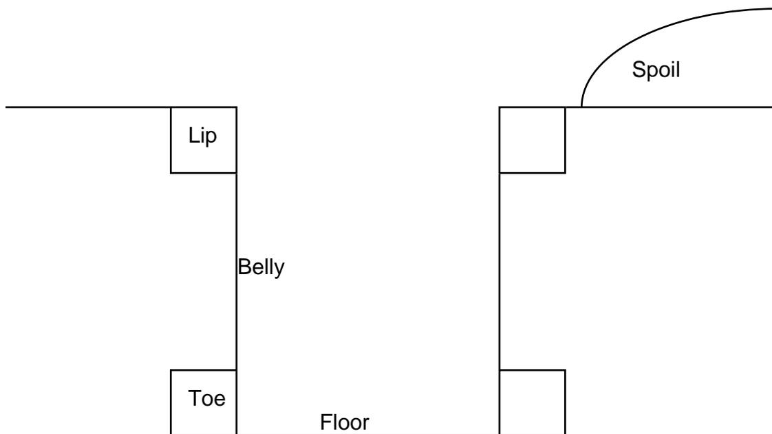
The **lip** usually refers to the area at the top of both sides of the trench, and the **toe** the area on both sides of the floor of the trench. The **belly** refers to the space between the lip and toe of the trench, and the **spoil** refers to the soil, rocks or other materials removed from the trench. The spoil pile must be at least 0.61 m away from the lip of the trench.
