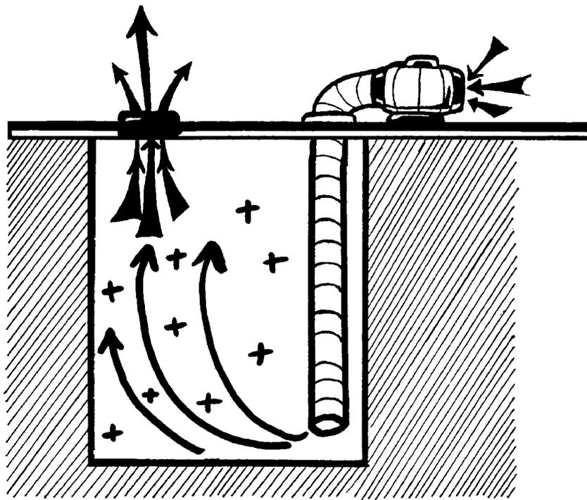
Addition of Duct Work to Avoid Short-Circuiting
