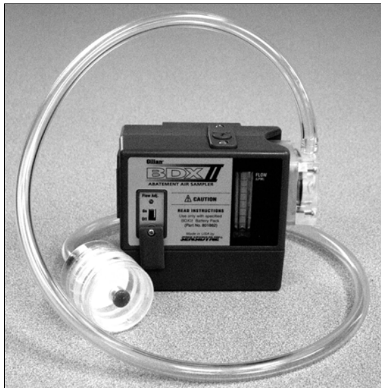
Personal sampling pump with a particulate filter or cassette.
