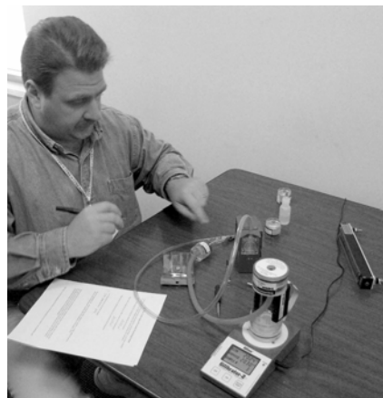
Union health & safety trainer factory calibrating a personal air sampling pump.
