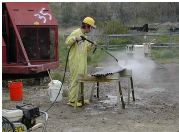
Figure 2: Cleaning of the Used Drill Steels with High-pressure Water.
