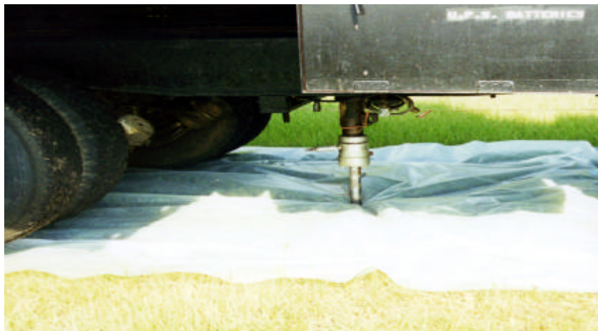
Figure 3: Cone Penetrometer truck used to deploy the CPOSS for subsurface characterization.
