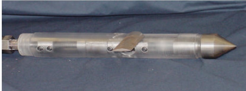
Figure 1: Cone Penetrometer off surface sensor tool with extended blades.
