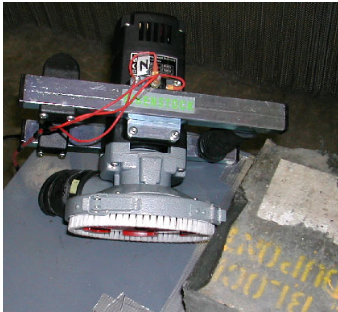
Figure 1: CS Unitec Grinder Model EBS 125D Next to Refractory Brick.
