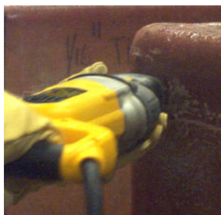
Figure 2. An operator using the DeWalt Reciprocating Saw to make a cut in the horizontal direction.
