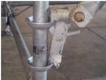
Positive locking trigger mechanism fastened to vertical bar.
