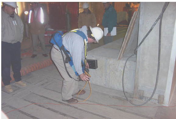
Figure 1: Operator using the GPR on a Vertical Concrete Surface.
