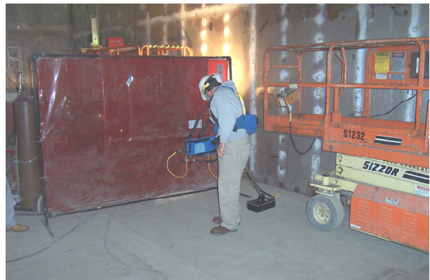
Figure 2: Operator using the GPR on Concrete Floor.
