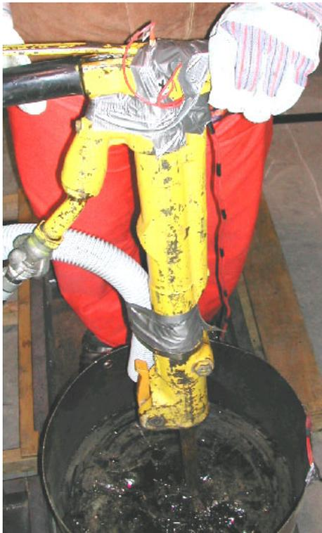
Figure 1: Ingersoll Rand Paving Breaker Model PB35AS8 Breaking Borosilicate Glass.
