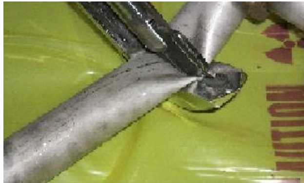
Piece of metal being cut by BPC-4.
