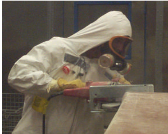
Figure 2. An operator maneuvering a corner with the Milwaukee Worm Drive Circular Saw.
