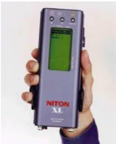
Figure 1: The NITON XL-309 Lead Paint Analyzer.
