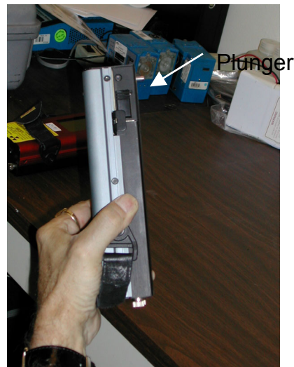
Figure 2: The Plunger Shows Whether the Shutter is Completely Open, Closed, or Partially Open for Safety Reasons.
