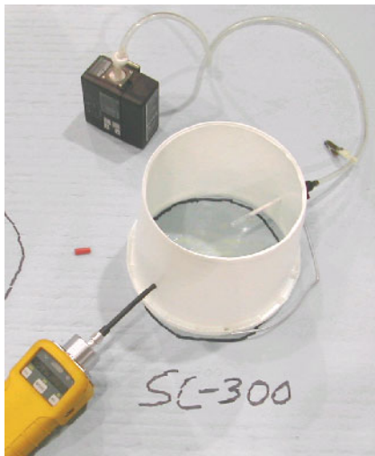
Figure 1: Assessment Configuration of PID and Air Sampling Pump on Concrete Substrate.
