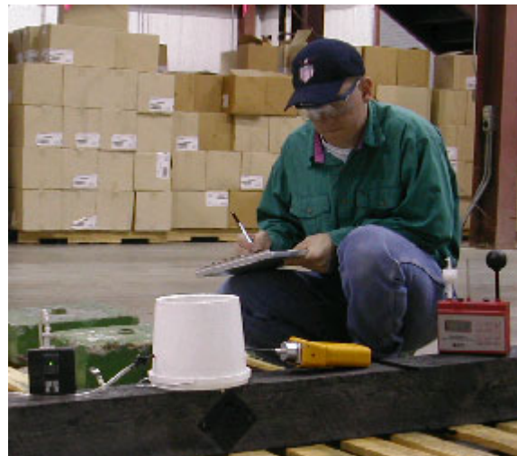
Figure 2: Assessment Configuration of PID and Air Sampling Pump on Wood Substrate.
