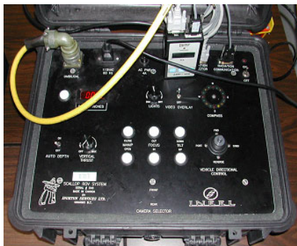
Figure 3: The RUCS Control Panel from Above.
