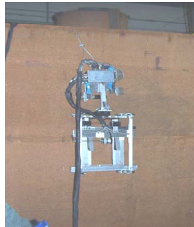
Figure 2: View of RONDE Crawler/scanning Bridge on Mock-up Tank Wall.
