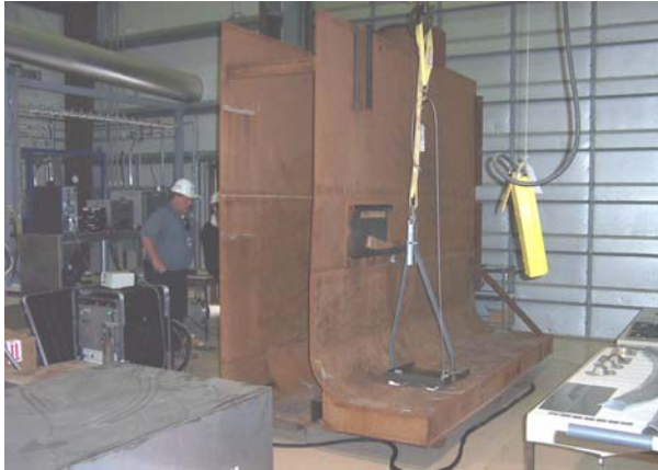
Figure 3: View of Tank Mockup with the Deployment Sled in Foreground on the Tank Bottom.
