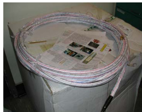
Figure 4: The NAPL Ribbon Sampler with indelible ink.
