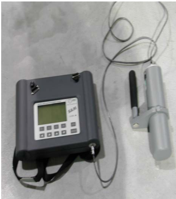
Figure 1: Complete SAMS Unit Showing the Console and the Sensor with the Ninety-Degree Handle.
