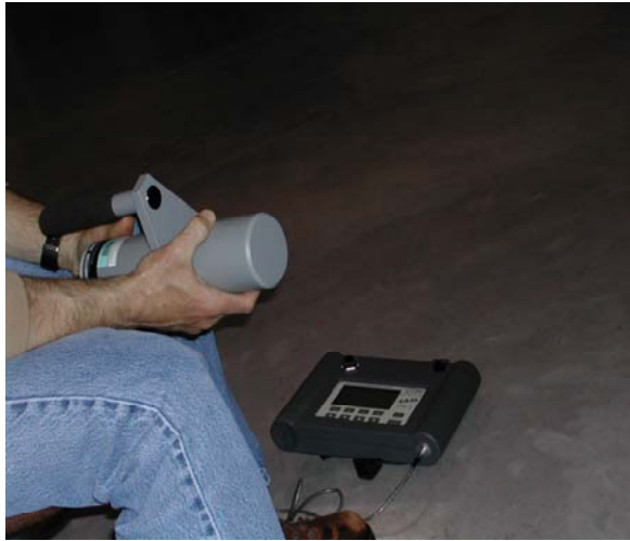
Figure 3: Technician Connecting Sensor to the Consol.
