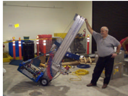
Figure 4. RadTrax without counterweight and survey head.
