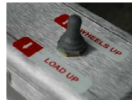
Figure 4: Ultra Lift Switch Used to Raise and Lower Both the Load and Wheels.
