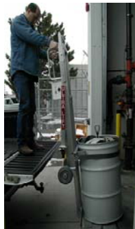
Figure 1: User Extends the Ultra Lift up to the Truck Bed
