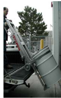
Figure 2: User Pulls the Load up Using the Screw Drive System
