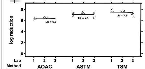
Peracetic acid/hydrogen peroxide (each point is a test; red line indicates the mean)
