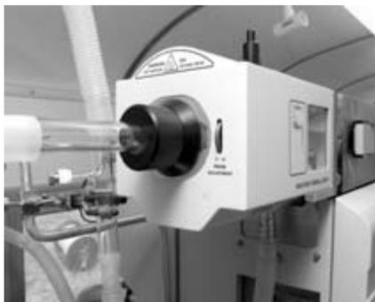
**Atmospheric Pressure Chemical Ionization (APCI) Source**
