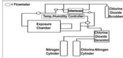
Generator: CDG Technology bench-scale chlorine dioxide generator, Model "Micro"
